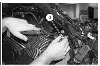
18. Remove the two bolts and continue prying the backbone rail upward until a large Phillips screw driver or steel rod can be inserted in the lower bolt hole to hold the end of the backbone rail up. This will give enough clearance between the backbone rail and the cylinder heads to remove the valve covers and the cams.
