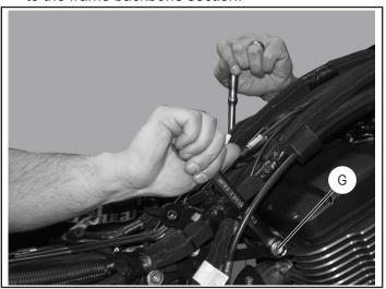
17. Insert a pry bar through the cut-out in the rear motor mount bracket. Pad the end with a shop rag to avoid damaging the paint, and pry upward on the rear end of the back bone rail to relieve any stress on the two bolts (G) that hold the bracket to the frame section.
