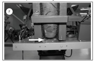
16. Using a 19mm socket and a 19mm box end wrench, loosen the three bolts (G) holding the rear motor mount bracket to the rear cylinder head and to the frame backbone section.
