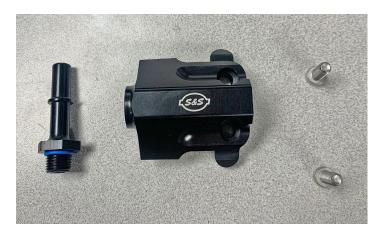
2. Install blue o-ring onto the fitting as shown
