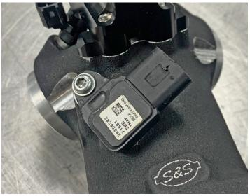
13. Install supplied screws with loctite and tighten
