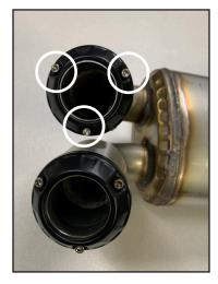
Remove supplied insert and replace with optional insert.
