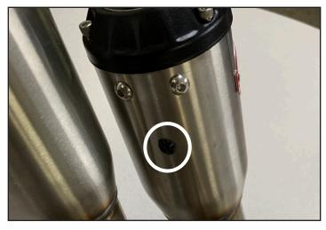
Take your 1/8 allen wrench and remove spark arrestor bolt
