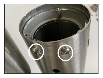
Remove the bulk head retaining ring.
