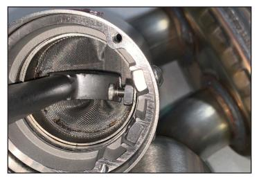
Remove the two bolts holding the retaining ring.
