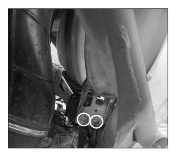
5. Remove the stock Muffler and keep in mind the right side aluminium rubber isolated block does not fall out.
