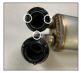
Tap the edge of the end cap with a dead blow or non marring hammer to pop it loose from the outlet tube.
