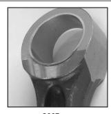
2007–up with stock pistons tapered crankpin boss -No Dots
