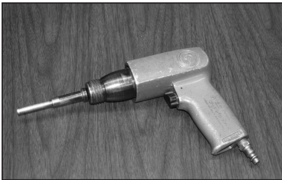
If a press is not available, guides may be removed and inserted with a valve guide driver and air hammer as shown
