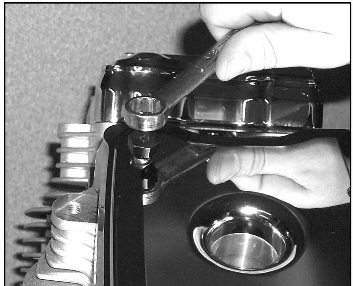
A 5/8" box or open-end wrench can be used where space limitations prevent use of torque wrench.
