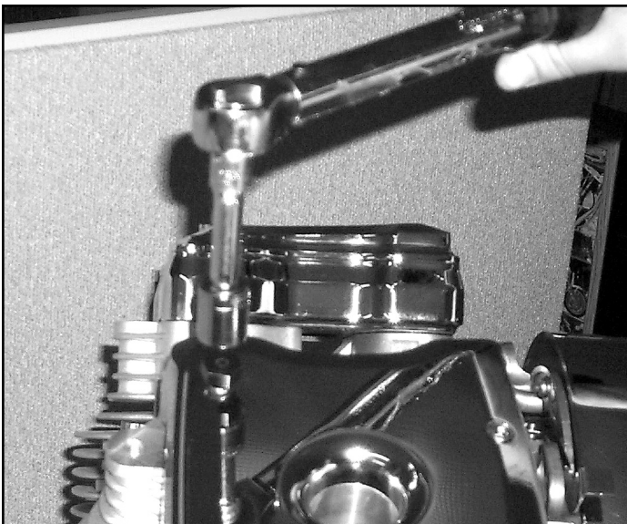
S&S® recommends use of torque wrench with rocker cover wrenches whenever possible.
