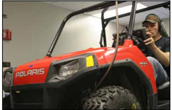
The chassis dyno provides a convenient way for our technicians to evaluate modifications to an engine installed in a vehicle. However, to get repeatable results the drive clutch had to be locked in high gear to avoid variations as the PVT changed gear ratios. This makes it somewhat difficult to use a chassis dyno in the field
