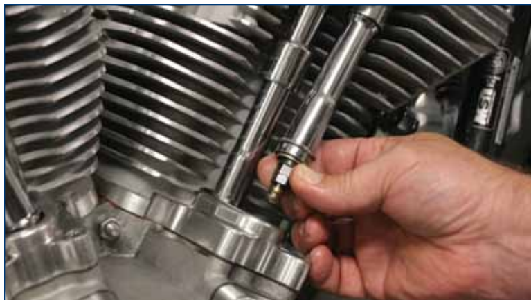
When a Quickee is collapsed, it can easily be installed or removed from an assembled engine.
