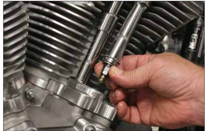
When a Quickee is collapsed, it can easily be installed or removed from an assembled engine.
