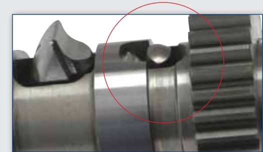
Increased rpm causes the compression release lobe to be centrifugally retracted so the engine runs normally.
