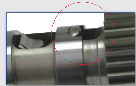
The compression release lobe reduces compression until the engine starts.
