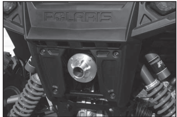
Picture 11 - Installed Exhaust
