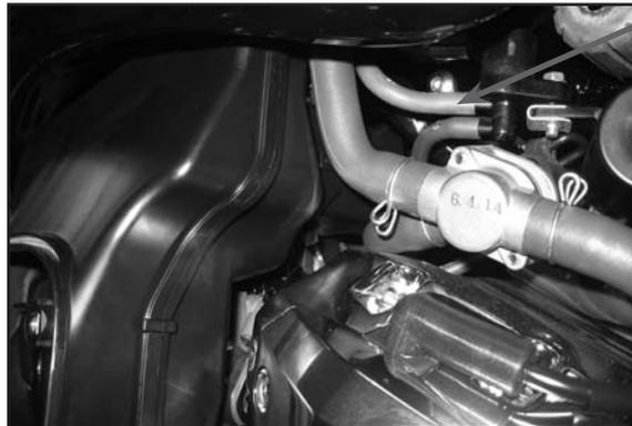
Remove hose, install rubber vacuum line cap on intake duct control solenoid fitting.
