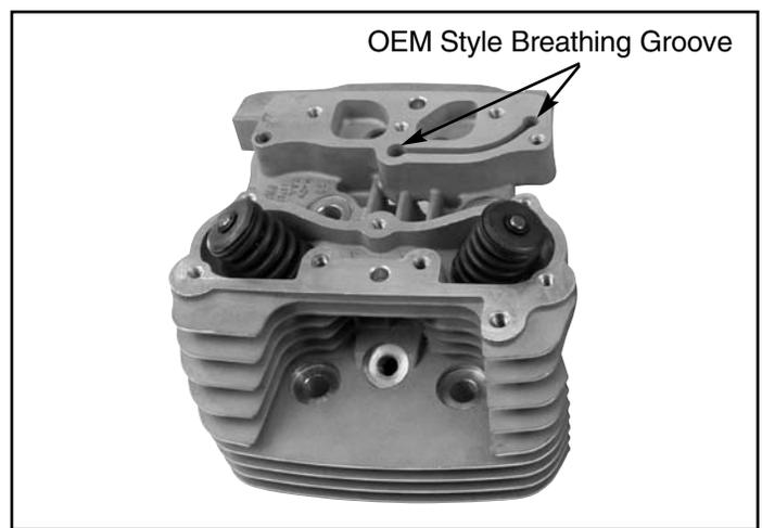
**Picture 2 - OEM Style Cylinder Head**
